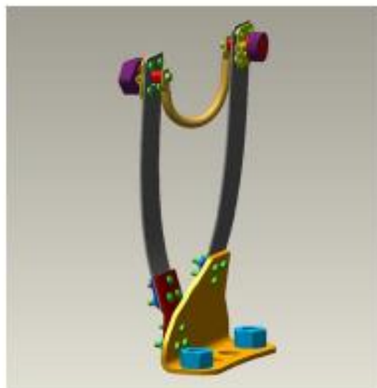
Figure 2-5: LCTU between blades and nacelle chassis
